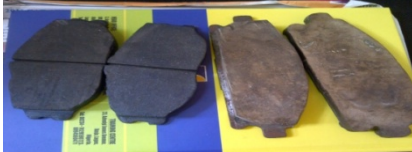
Produced sawdust composite brake pads
